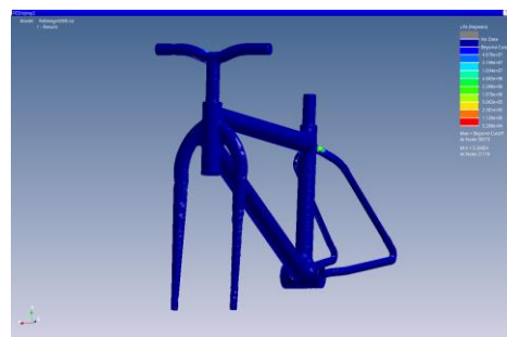
Figure 15 Redesigned Frame Strain-Life Prediction
