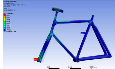
Figure 24 Scenario 3b Titanium frame Von-Mises Stresses under (50/50) load distribution
